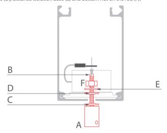
**4.** Insert the rod from the fixture through head.
