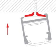
**NOTE!** Unusual dismounting of the extrusion. Move the extrusion in one of the directions in the horizontal plane, gently pull one side of the extrusion down, and remove the extrusion from the brackets.
