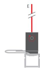
**9.** Attach the light fixture with the arm (E) to the top head (F). Block the arm by tightening the pressure screw in the top head with the Allen wrench.
