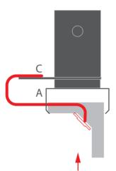
**2.** Insert the rod into the mounting bracket of the head (D). Block the rod by tightening the pressure screw in the head with the Allan wrench.
