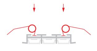
**2.** Insert the extrusion into the groove bending the spring arms towards each other.
