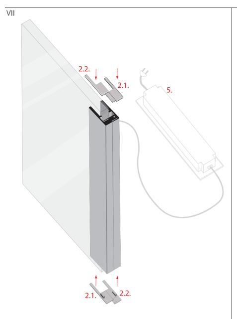
Put both end cap parts on both ends of the profile. First insert item (2.1), then item (2.2).
