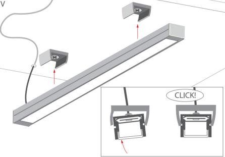
Connect the power and insert the lighting fixture into the mounting brackets.
