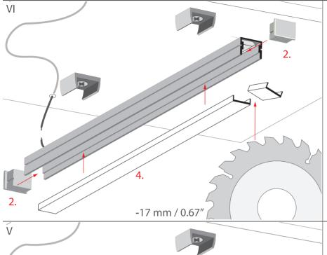
Cut the cover (4) so that it is 17 mm / 0.67" shorter than the extrusion.
