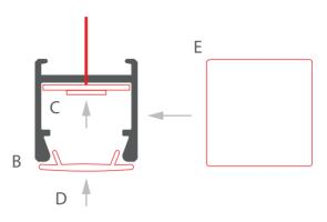
**3.** Connect power to the LED strip and mount the extrusion (B) in the mounting brackets (A).
