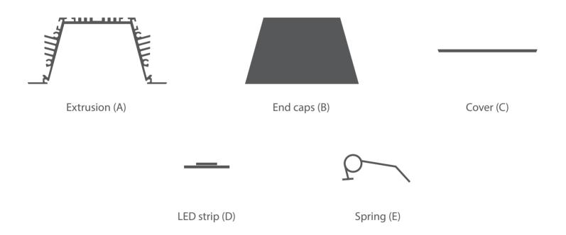
**NOTE!** All LED strips must be connected to a 12 V or 24 V power supply.
