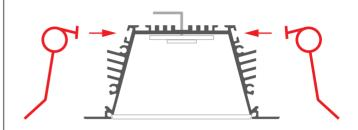
${\bf 3.}$  Connect power. Pull the springs inward and insert the extrusion (A) into the mounting groove.
