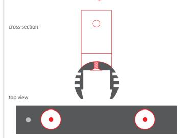
**3.** Mount the LED strip in the extrusion and lead the cable through a pre-drilled hole.
