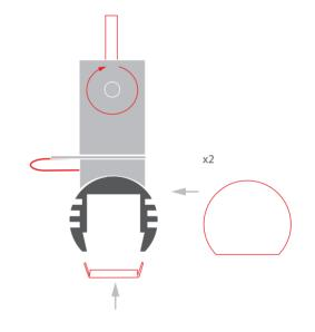
**5.** Install the W-KG-Z ceiling fasteners. The fastener installation manual can be downloaded at www.klusdesign.eu. Connect the cables, each for the single power pole to the fasteners. The cables should go through a pre-drilled hole just under the masking cover of the fastener.
