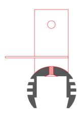
**3.** Mount the LED strip in the extrusion and lead the cables through pre-drilled smaller holes. Then lead them to the connector sof the DP-ZZ-PDS-O fasteners. Each hole should lead a cable with one power pole, LED strip has to be cut before installation, so the wires can be easily routed to the holes.
